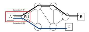
Both requests will go through quantum repeater R. The network needs to manage and orchestrate servicing both of these connections simultaneously by gauging resource usage, resource optimization, and multi-tenancy.
