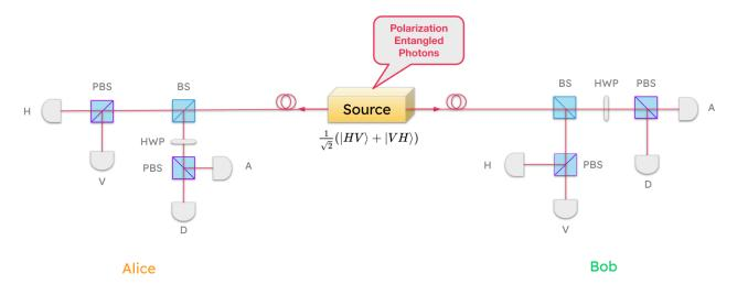
At the center is the entangled photon source. It's generating pairs of polarization-entangled photons at very high rates. One photon of the entangled pair is sent to Alice and the other photon of the pair is sent to Bob over some fiber. Alice and Bob have essentially the same set of hardware for measuring the quantum state.
