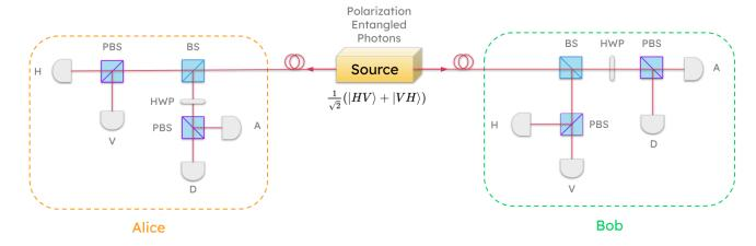
Pictured above is a hardware schematic for a polarization-encoded BBM92 network. This is BrightNet, a quantum network that was built at Aliro headquarters in Boston.
