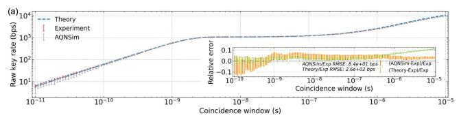
A coincidence window is the time bin used to identify clicks at end nodes as pairs of entangled photons. As the coincidence window widens, more true pairs are identified, so the raw key rate rises. Make the window too wide, and uncorrelated clicks (accidentals) will be counted, falsely inflating the raw rate.
